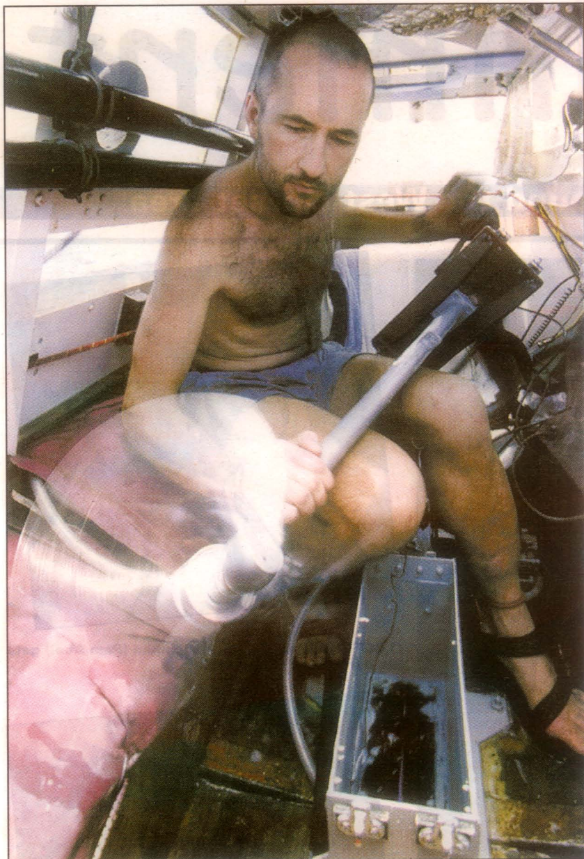
□ Showing the propulsion mechanism a 16 inch stainless steel propeller with a 6:1 pedal ratio mechanism capable of 400 rpm.
