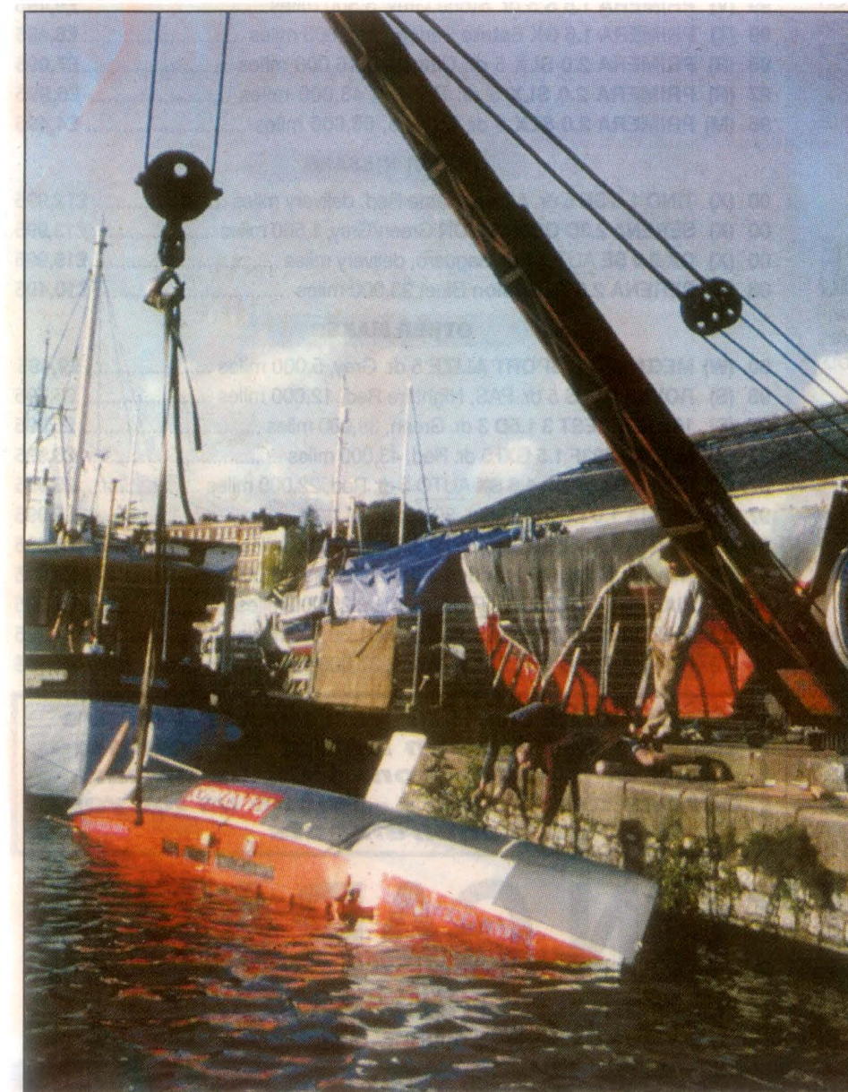
BELOW: Testing that a capsized Moksha could be righted at Exeter Maritime Museum - a precaution that was to prove essential after a curious whale upturned the boat in the middle of the Atlantic at 3am
